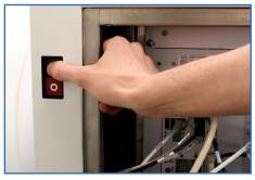
Turn on the power console and wait at least for 30 sec. Note: This will automatically reactivate the SampleJet.
