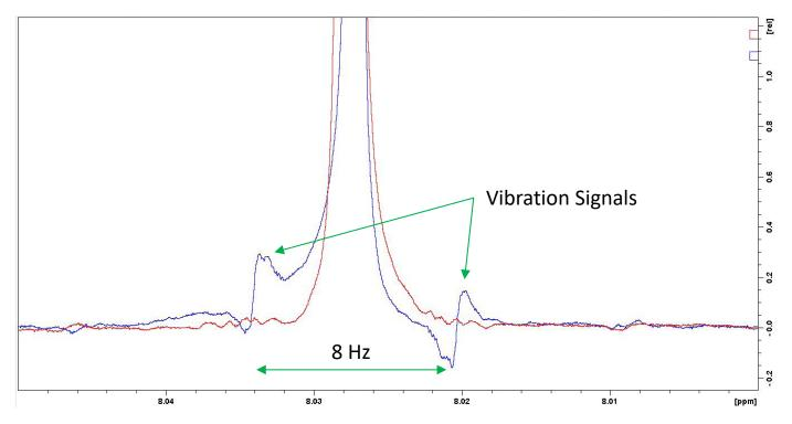
Figure 1: Overlay of a maintenance spectrum with vibrations (blue) and without (red) vibrations. The vibrations can be seen as peaks at +/- 4 Hz around the main signal.
