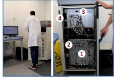
Open the NMR console. Switch off all units from bottom to top (1-3). Give each unit time to shut down completely to avoid any system errors. Then turn off the console power (4).
