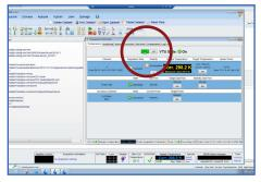
Open the TopSpin Software and switch on the vtu temperature control. Wait until temperature display is green.
